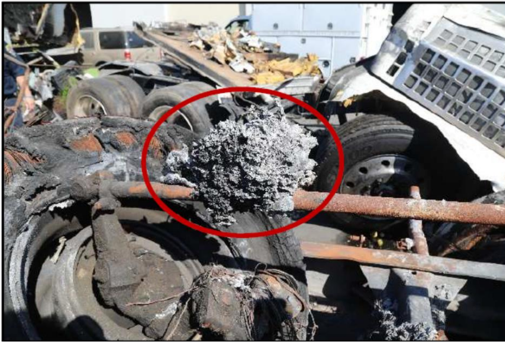
Figure 17. Melted ECU on steering linkage.
