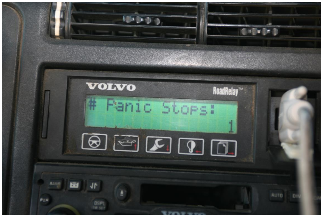
Figure 6. Cummins RoadRelay3 trip computer Panic Stops Counter.
