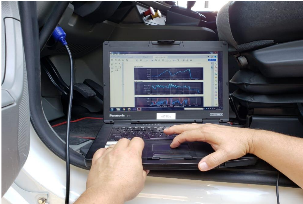
Figure 3. Cummins PowerSpec software connected laptop via J1939/13.
