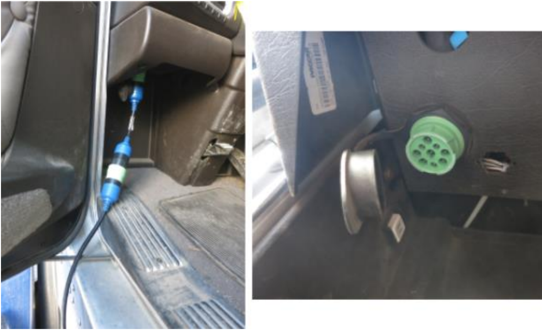
Figure 13. SAE J1939-13 Type II 9-pin Deutsch connector (green).
