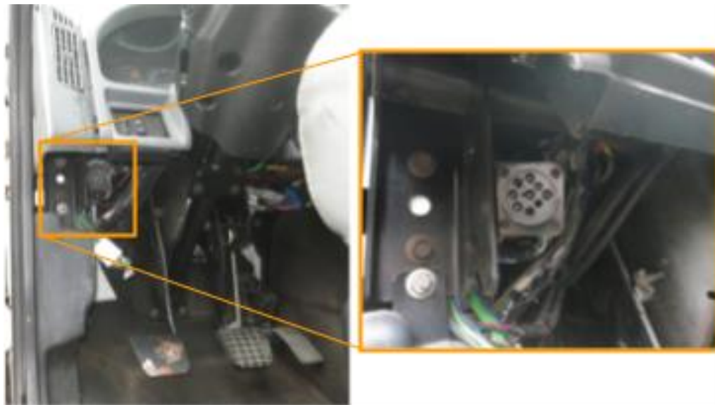
Figure 12. SAE J1939-13 Type I 9-pin Deutsch connector (black).
